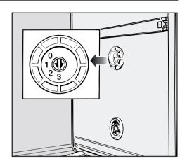
■ Use a coin or screwdriver to adjust the water hardness level selector in the wash cabinet. There is a click as each setting is reached.
